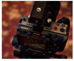
x 2160) output, delivering 4K movies with overwhelming resolution. The image sensor maximizes light collection efficiency so that clear, usable images can be captured even in challenging low light. Standard ISO sensitivity is 100 to 32000, and latitude is an impressively wide 14+ stops when recording in S-Log3 gamma.
